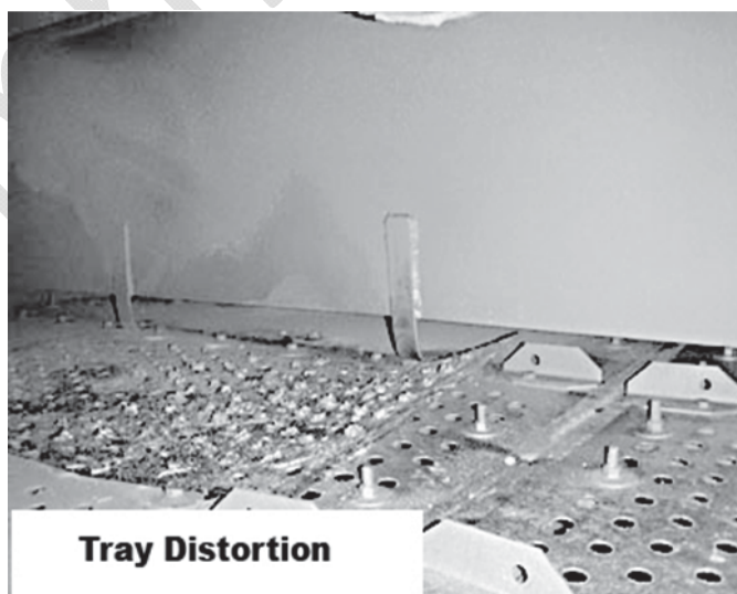
Figure B.4 - Sieve Tray Distortion
