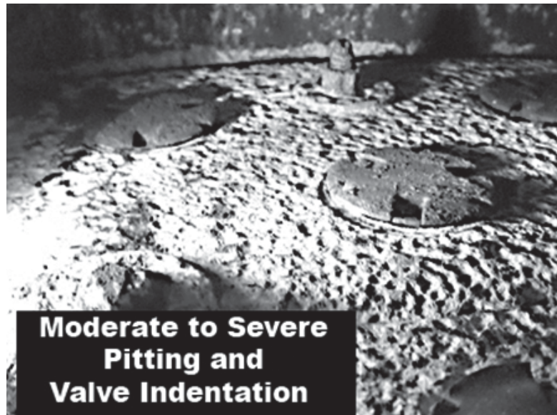
Figure B.66 - Indentation of Valves
