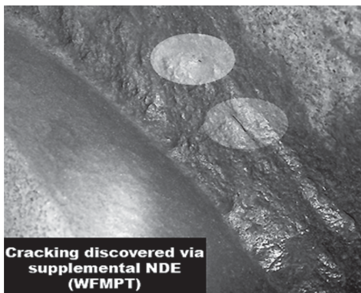
Figure B.56 - WFMT Discovered Cracking
