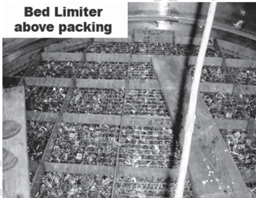
Figure B.43 - Bed Limiter Above Random Packing
