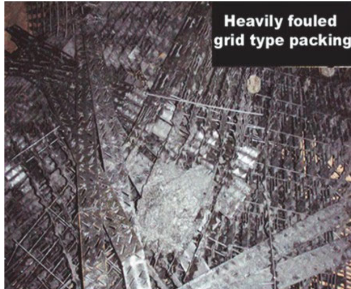
Figure B.49 - Fouled Grid-type Packing
