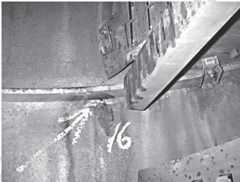
Figure B.87 - Breaching of the Seal Weld
