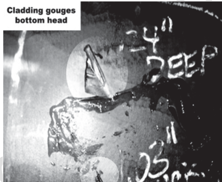
Figure B.52 - Cladding Breech at Gouges in Bottom Head
