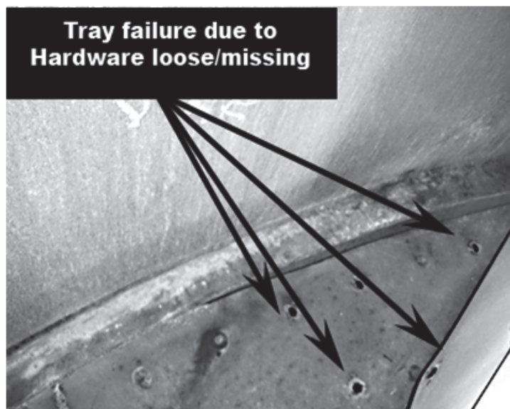
Figure B.78 - Loose and Missing Hardware Failure
