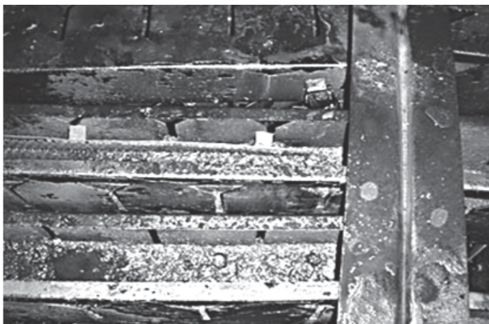
Figure B.38 - Fouled Troughs on Box and Trough Distributor
